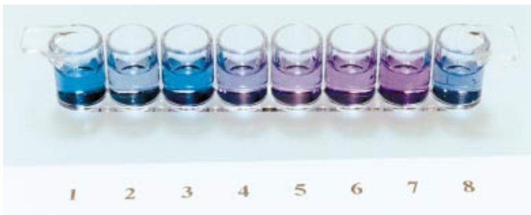
Figure 10. PNA/DNA hybridization induces a blue–purple color change: well 1, no PNA or DNA; well 2, 600 pmol (3.0 \mu M) of DNA; wells 3–7, 600 pmol of PNA + 0, 150, 300, 450, and 600 pmol of complementary DNA; well 8, 600 pmol of PNA + 600 pmol of noncomplementary DNA. The complementary PNA + DNA strands formed the hybrid PD2 (Chart 1), while the noncomplementary DNA strand used in well 8 had the sequence 5'-CGATGATGATC-3'. All samples contained 15 \mu M DiSC 2 (5) .
